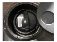
will prevent the pumps from getting air-locked at initial start-up. If the pump does get air-locked, loosen the bleeder value on top of filter, release air. This may need to be done several times for pump to start to move water.
